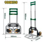
Load capacity: 100kgs Frame material: aluminium tube Foot plate material: steel Extended size: 400x385x1000mm Folded size: 60x385x640mm Foot plate size: 265x385mm Wheels: 125mm(PP+ TPR) Including elastic bungee cord Compact design, easy to store almost a
