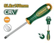
Tip type: slotted Tip size: 8.0mm Round shank Diameter: 8.0mm Length: 150mm Material: Cr-V steel Blade finish: black tip Magnetised tip Comfortable soft grip handle Packed by plastic hanger
