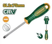
Tip type: slotted Tip size: 3.0mm Round shank Diameter: 3.0mm Length: 75mm Material: Cr-V steel Blade finish: black tip Magnetised tip Comfortable soft grip handle Packed by plastic hanger
